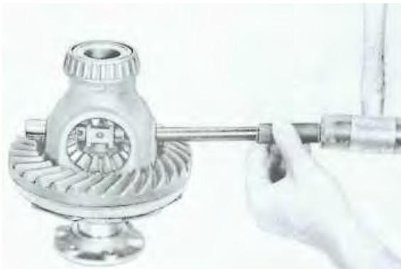
3. Turn the pinions so that the small pinions can be taken out through the side openings in the differential housing. Remove the large pinions together with the threaded lock pieces.
