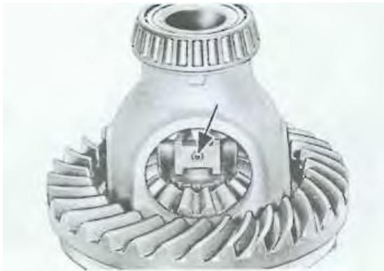
2. Remove the shaft with a punch and take out anchor piece.
