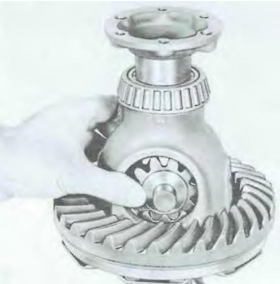
5. Insert the small differential pinions through the opening of the housing. Position them opposite each other so that their bores align with the bores of the housing.
