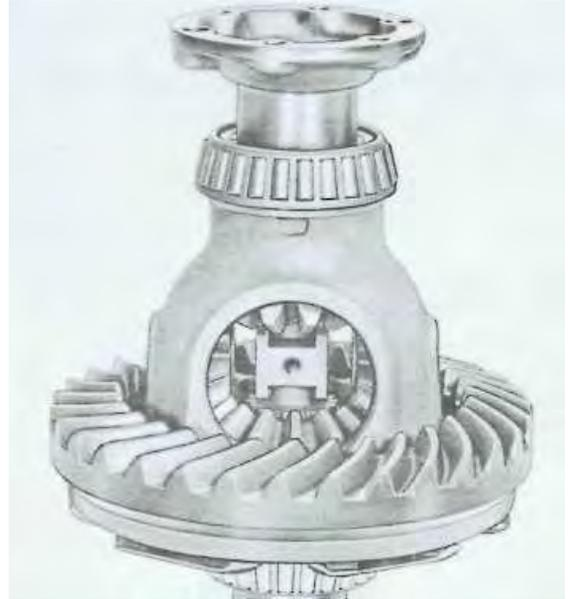
7. Install the pinion shaft while holding the anchor piece thereby preventing the anchor piece from binding on the shaft during installation.
